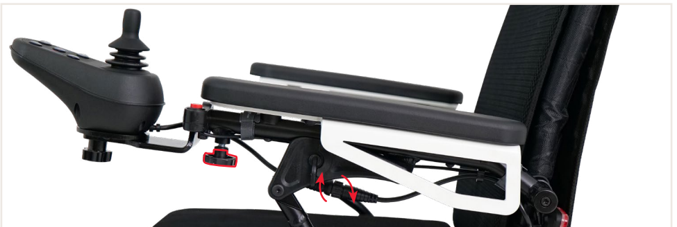
Image 6: Fixing and connecting the operating module
