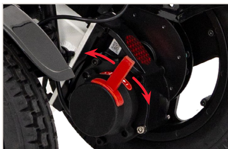
Image 14: Activating or deactivating the parking brakes
